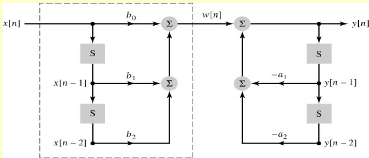
Block diagram of A second-order difference equation. (Direct form I : needs 4 memory locations:
