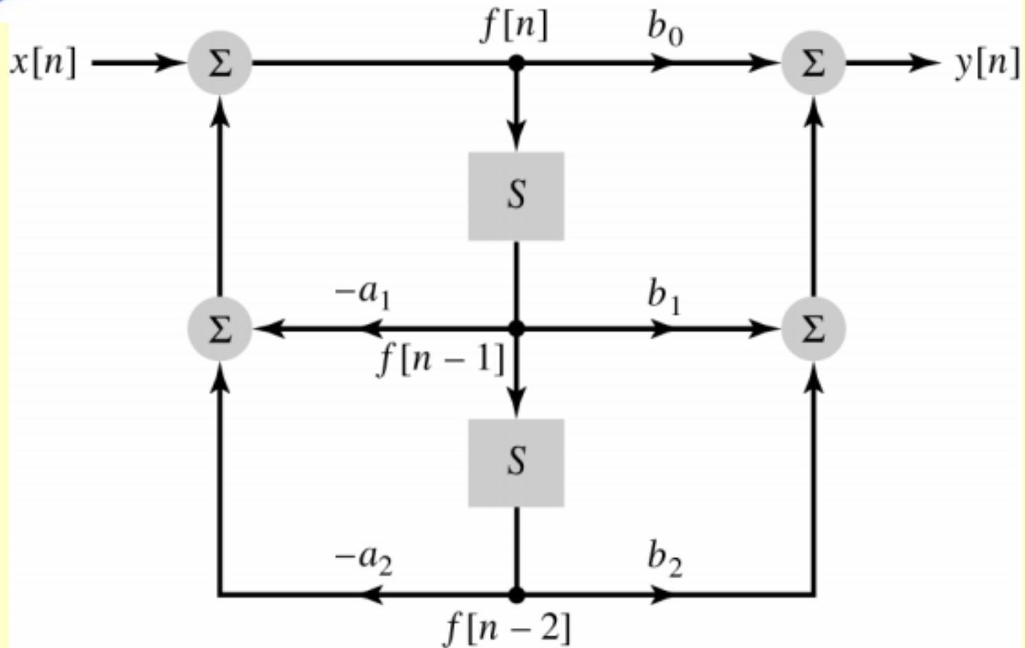
Block diagram of A second-order difference equation.
