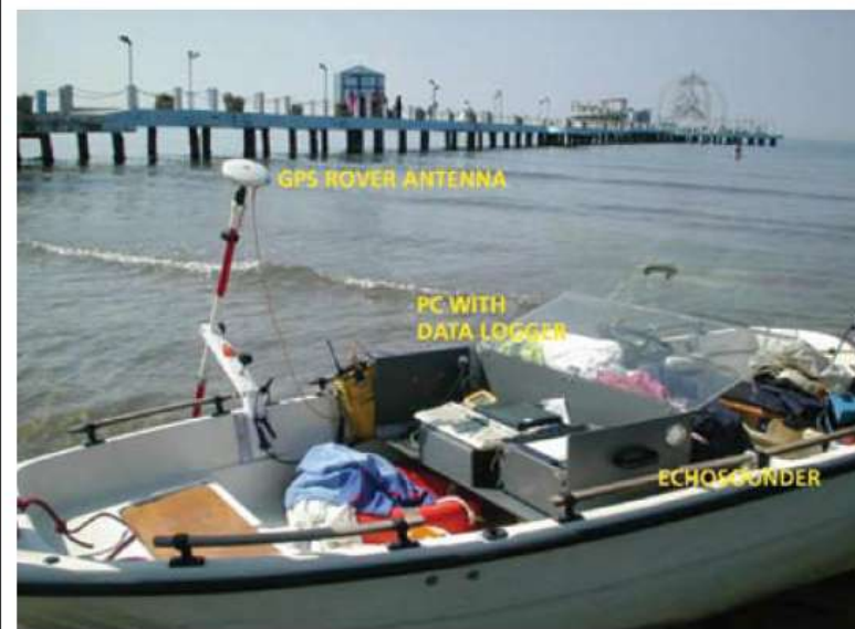
FIGURE 12 Typical small vessel outfitted for hydrographic surveys
