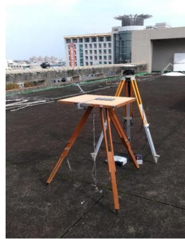
Fig. 2. Simultaneous GNSS observations collected by PP6 and Mi8
